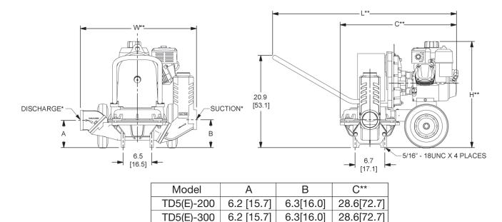
\*\*This dimension may vary due to engine manufacturer's specifications. NOTE: Dimensions are in inches (centimeters) and have a tolerance of +- 1/8".
