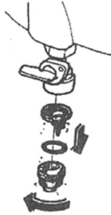
Fuel Filter Element Removal
