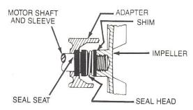
Figure 2 - Shaft Seal Replacement
