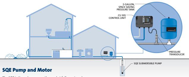
The SQE is the only pump on the market fully equipped with built-in electronic controls which allow for advanced computer controlled performance and state of the art protection features including sophisticated diagnostics. The motor design is a Variable Speed Drive which electronically changes the pump speed to match demand providing you with the incredible comfort of constant pressure.
