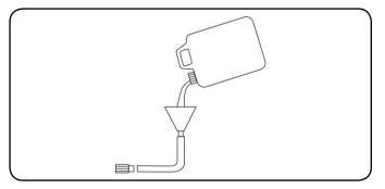
5. Pour the antifreeze into the funnel, then pull on the engine recoil starter to create suction in the pump housing. Pull the recoil several times until antifreeze comes out of the pump outlet.
