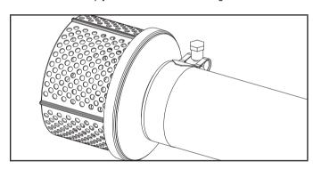
20. Tighten the clamp to 7.4±1.5 lbf-ft (10±2 Nm) with a 10mm wrench. If you do not have a torque wrench, hand tight then ¼ turn past full tight.
