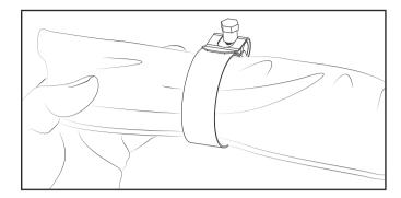
4. Slide the blue discharge hose over the outlet hose fitting.
