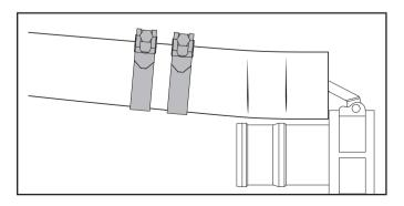
7. Insert the threaded or quick coupler in the green rigid suction hose until properly seated.
