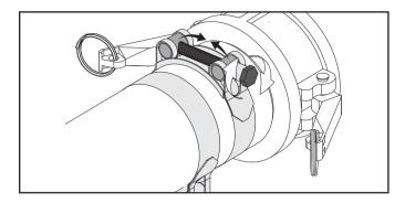
11. Test connection is tight by twisting coupler in the hose to make sure it doesn't turn. If coupling turns, then tighten clamps further until coupling won't turn.
