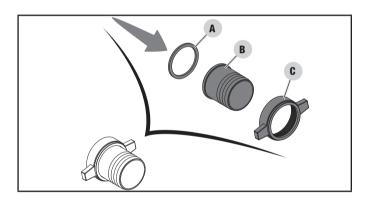
2. Thread the assembled connector to the outlet fitting (top of pump). Locate the blue "outlet" label on the pump.
