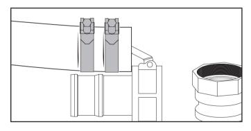
6. Slide the clamps back and start to assemble the green hose to cam lock coupler.
