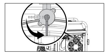
3. Move the choke lever to the "CHOKE" position by pulling out.
