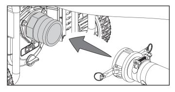
15. Lock in place with the cam levers.
