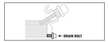
2. Allow the oil to drain completely into an appropriate container.
