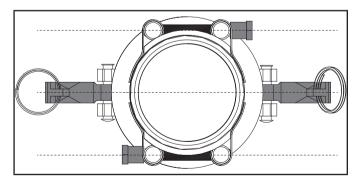
10. Tighten each clamp to 7.4±1.5 lbf-ft (10±2 Nm) with a 10mm wrench. If you do not have a torque wrench, hand tight then ¼ turn past full tight.
