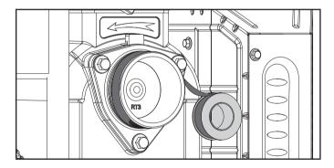
13. Thread the fitting over the tape and hand tighten. If you have channel locks large enough, you can give it a ¼ turn past hand tight.
