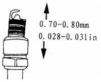
4) Check the plug O-ring for normal condition. Screw it in with the plug wrench to protect the plug thread.
