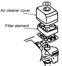
1) Unscrew the wing nut and remove the air cleaner cover and filter element.
