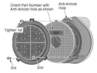
Assemble Screen and Shield as shown.
