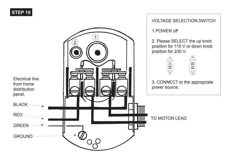
We recommend that a licensed electrician be employed to do wiring to the pressure switch. Permanently ground the motor in accordance to the electrical codes for your area.
