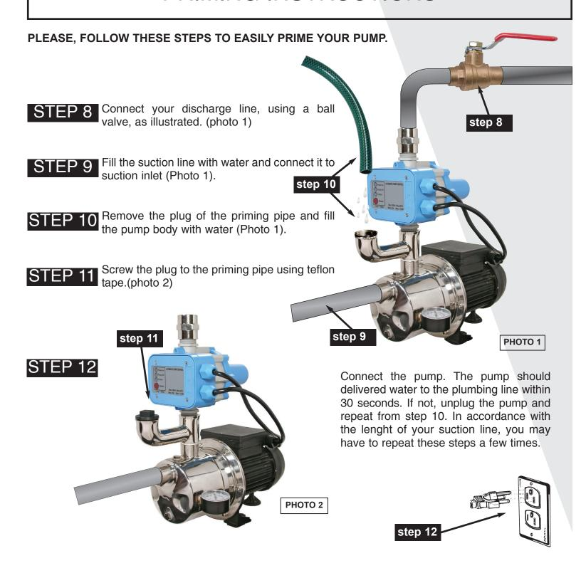
NOTE: After installation, if the pump is cycling "on-off" and/or comes on when you are not visibly using water, the pump is not defective. It means you have a leak on the discharge side of the pump. The leak must be localised and needs to be repaired. If you need assistance to determine same, please call 1-800.361.1820. The pump is warrantied by the manufacturer and you must call us to determine procedures. The pump cannot be returned to the point of purchase without our prior consent.
